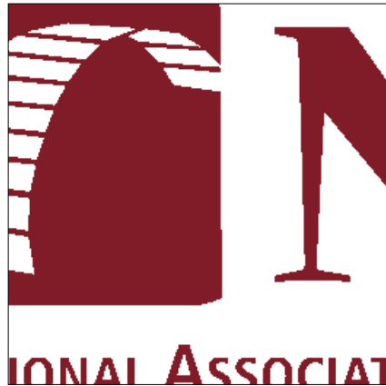
NAILBA logo as TIFF raster file, greatly enlarged. Notice the “bitmapping” of the edges.
